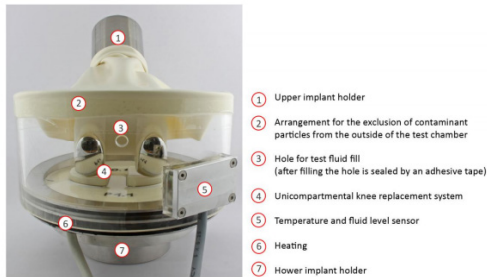
Fig. 7: A representative test chamber.
